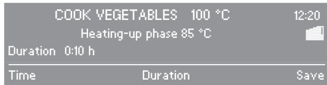
As soon as the set temperature has been reached, "Heating-up phase" will disappear from the display. The cooking phase will now begin and the duration will start counting down.
